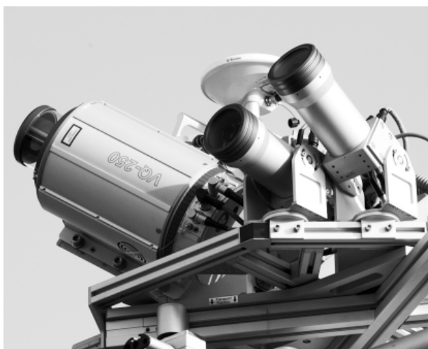
Fig. 5: mobile laser scanning system RIEGL VMX-250 with the modular camera system VMX-250-CS6
