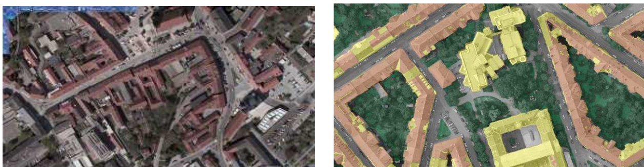
Figure 3: UltraCam image (left) and classification map (right), derived automatically from the image.
