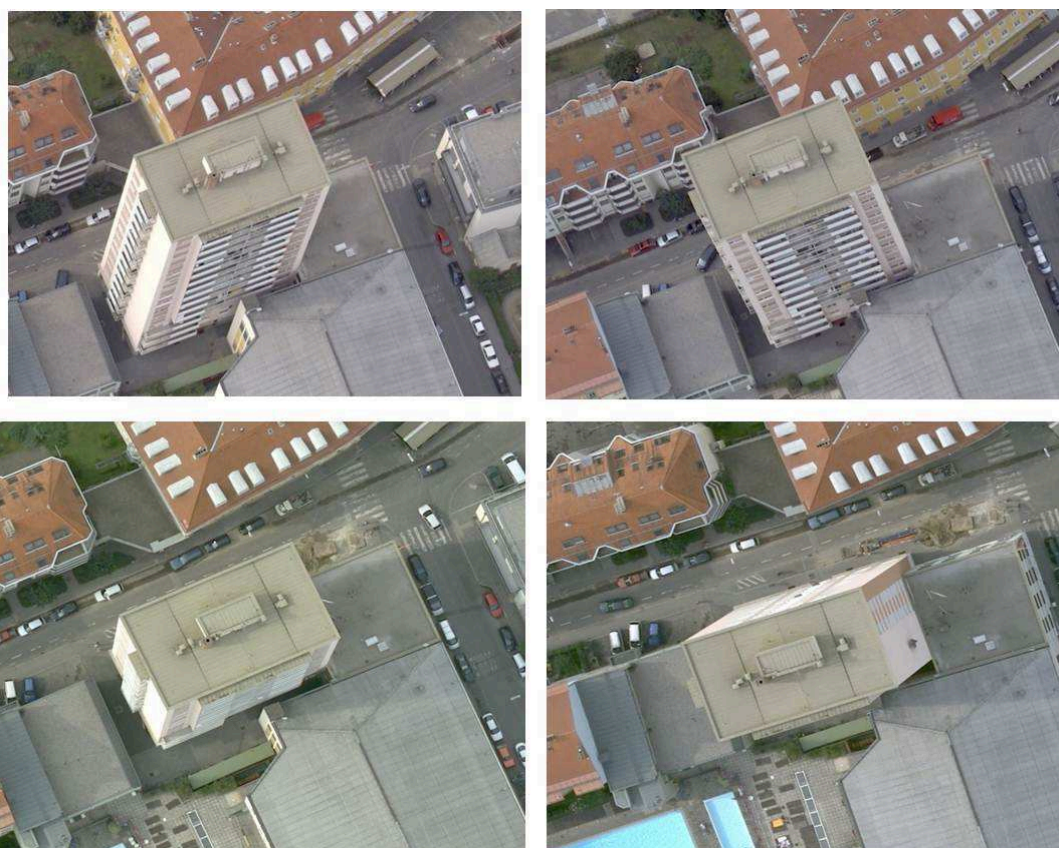
Figure 1: Multi-ray photogrammetry is the underlying methodology for Microsoft 3D city model generation. Specific flight pattern ensures redundancy and avoids occlusions
