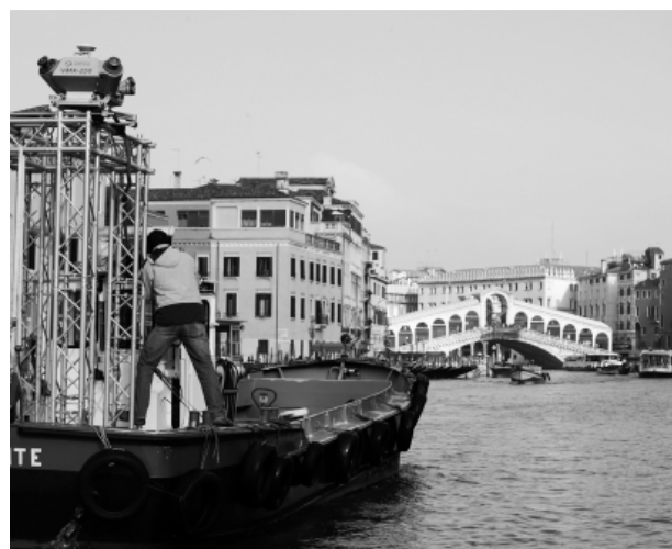
Fig. 6: VMX-250 laser scanning system mounted on the workboat "Sante" while scanning the Grand Canal in Venice
