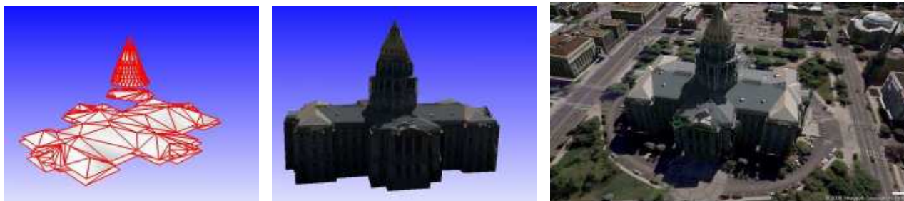
Figure 5: Automatically extracted roof polygon (left), extruded and textured vector building (middle) and global scene with the vectored 3D building model.
