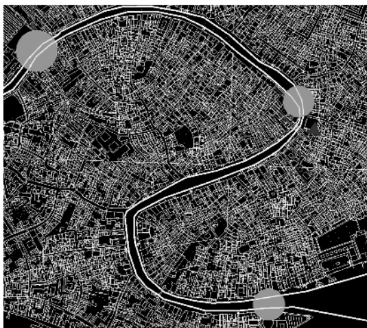
Fig. 1: CAD plan of Venice white: planned trajectory gray: areas with planned control points
