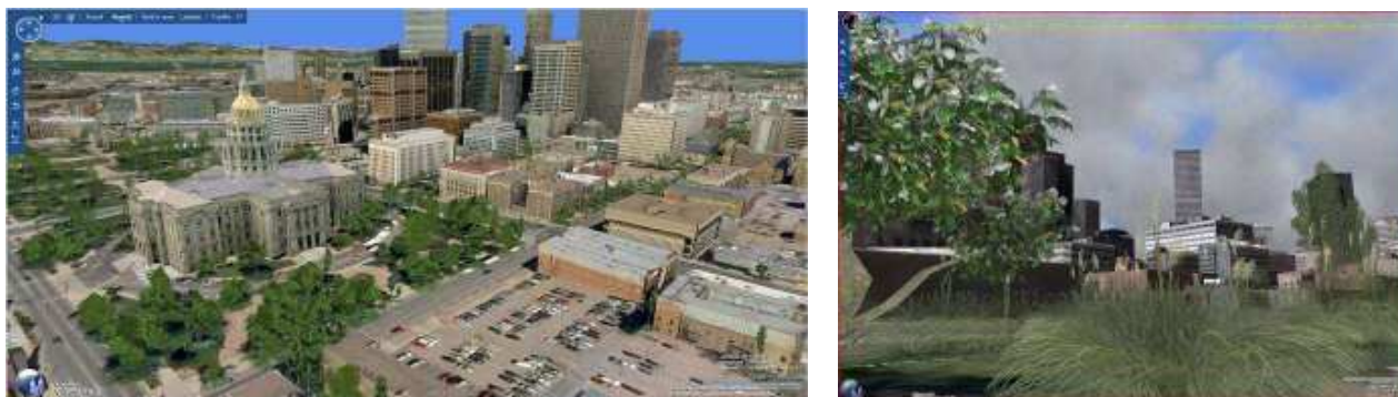
Figure 6: Examples of 3D city models in Virtual Earth, generated by the automated workflow based on multi-ray photogrammetry and UltraCam aerial images.
