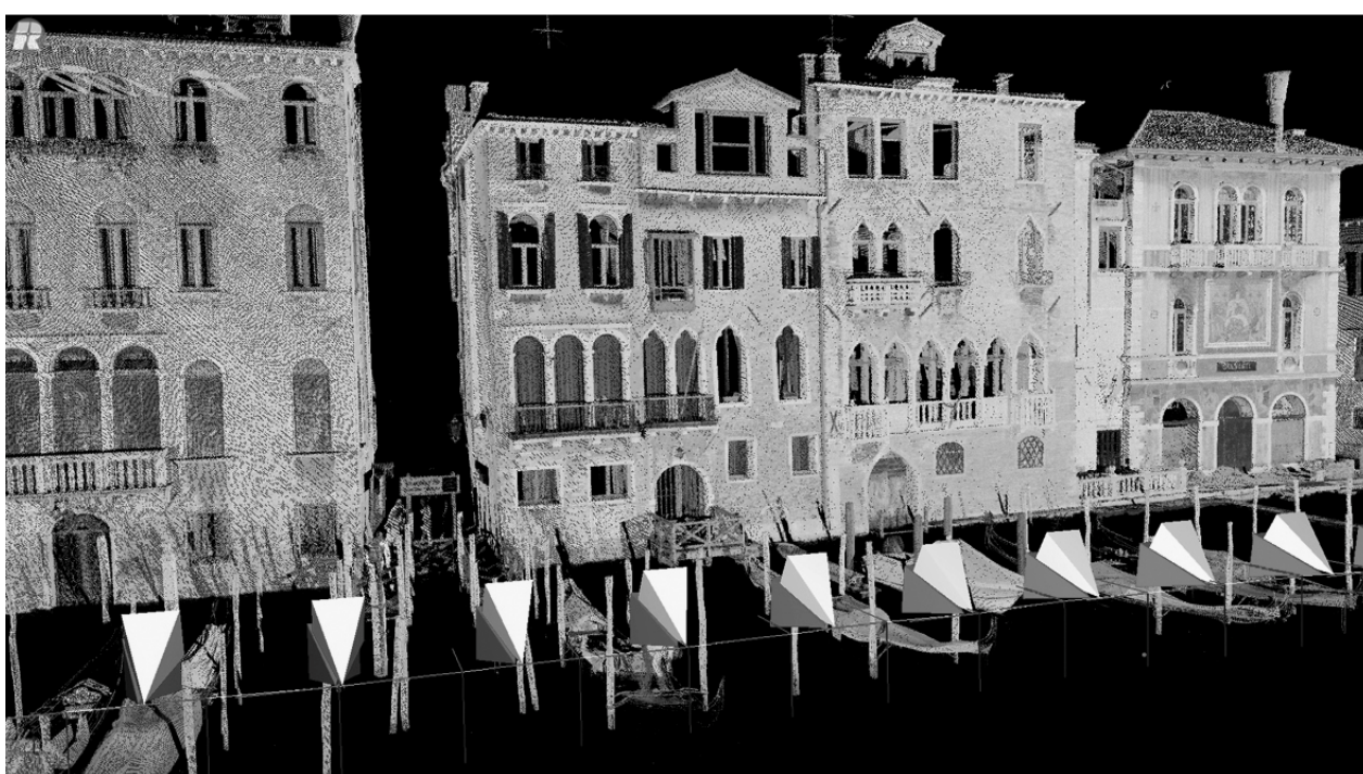
Fig. 4: Illustration of the camera positions and fields of view at the moment of their synchronous triggering. Light and dark gray cones represent the fields of view of camera 1 and 2 respectively. Scan data is displayed colored with the gray scaled relative reflectance [Rieger (2010)]
