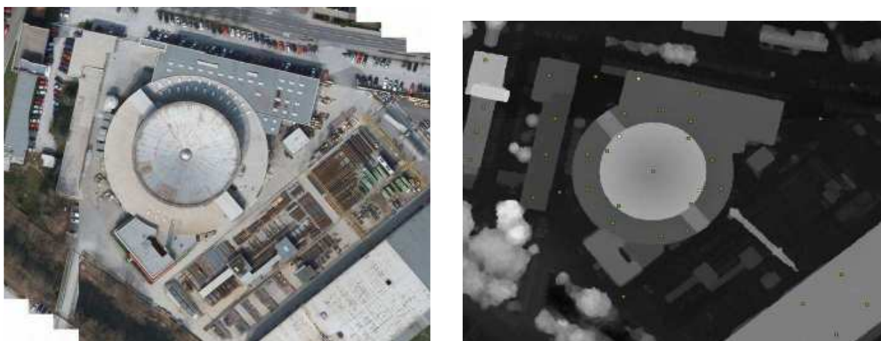
Figure 2: Highly overlapping UltraCam images (left) with 10cm ground sample distance and high resolution DSM (right), processed by dense matching from the images. Point density of the DSM is around 50 points per square meter, accuracy is better 10 cm.
