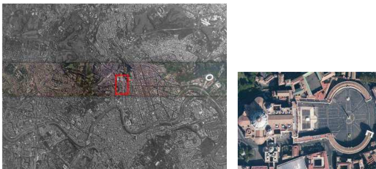
Figure 15: UltraCamG frame, Rome, Italy. Shows is oen full frame PAN and one RGB strip. The detail shows the Vatikan. Image resolution is 30cm.
